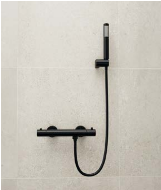
Brass mixer body matt black Thermostatic cartridge Vernet sensor 1,5m shower hose PVC anti-twist Anti-burn systems
